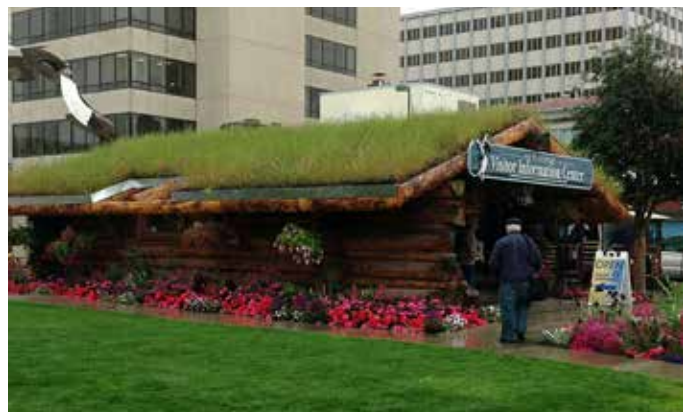
Above: Traditional Alaska cabins have often used 'green roof' systems, back when roofing materials were scarce and grass sod was the best protective and insulative material available.
